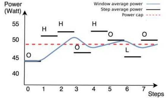
**Figure 5: Example of fluctuations of configurations performed by the enhanced strategy in-between different exploration procedures. Window size is set to 8. O denotes the configuration  $(p, t)^*$ , H the configuration  $(p, t)^H$  and L the configuration  $(p, t)^L$ . These configurations are fixed along each window but their power consumption could change.**
