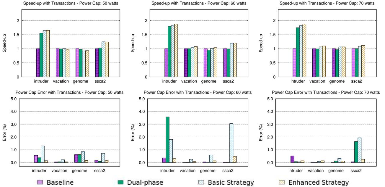
Figure 7: Speed-up and power cap error with transactions
