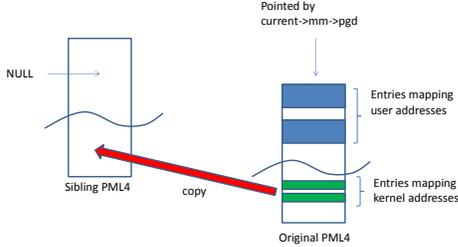
Figure 3. Initial setup of the sibling PML4.
