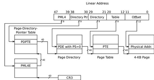
Figure 2. The paging scheme in `x86_64` processors.
