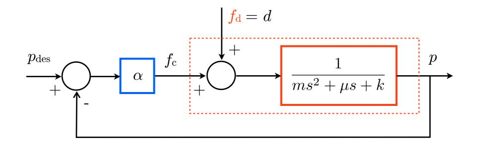
same feedback  $f_c = \alpha(p_{des} - p)$  as before, independent from the value of the disturbance since it reacts to the **effect** of the disturbance on the system
