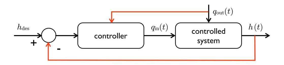
note that even if the disturbance measurement device has some malfunctioning the feedback will take care of attenuating the effect of the disturbance
