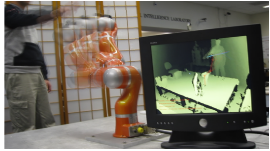
Fig. 2. Multiple overlapping image frames of the attached video showing the performance of the new collision avoidance strategy.
