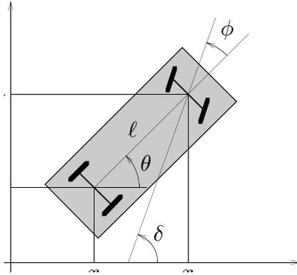
**Fig. 3.** Generalized coordinates of a car-like robot
