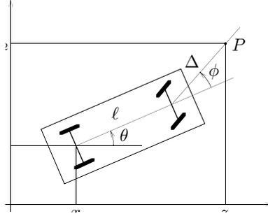
**Fig. 8.** Alternative output definition for a car-like robot
