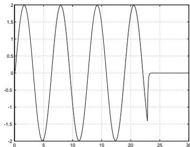
**Fig. 28.** Point stabilization with time-varying feedback and heat function  $\eta_4$ :  $x$  (m) vs. time (sec)
