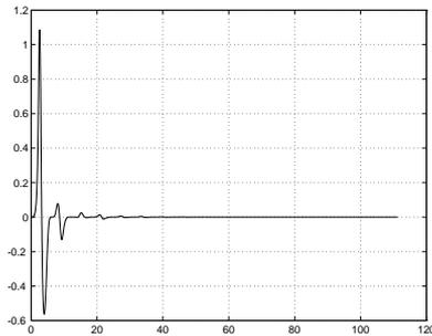
**Fig. 45.** Point stabilization with nonsmooth time-varying feedback (II):  $\phi$  (rad) vs. time (sec)
