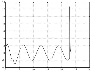
**Fig. 32.** Point stabilization with time-varying feedback and heat function  $\eta_4$ :  $v_1$  (m/sec) vs. time (sec)
