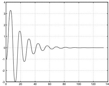
**Fig. 35.** Point stabilization with nonsmooth time-varying feedback (I):  $x$  (m) vs. time (sec)
