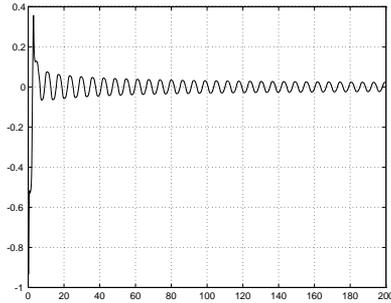
**Fig. 23.** Point stabilization with time-varying feedback and heat function  $\eta_2$ :  $\theta$  (rad) vs. time (sec)
