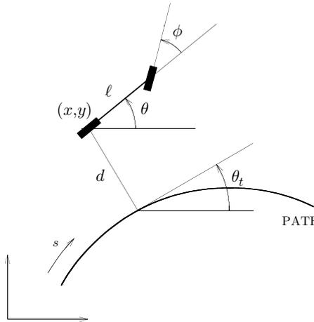
**Fig. 4.** Coordinate definition for a path following task
