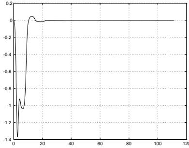
**Fig. 43.** Point stabilization with nonsmooth time-varying feedback (II):  $y$  (m) vs. time (sec)
