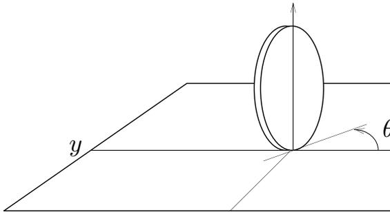
**Fig. 2.** Generalized coordinates of a unicycle
