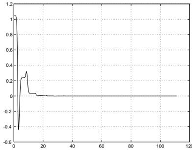
**Fig. 44.** Point stabilization with nonsmooth time-varying feedback (II):  $\theta$  (rad) vs. time (sec)
