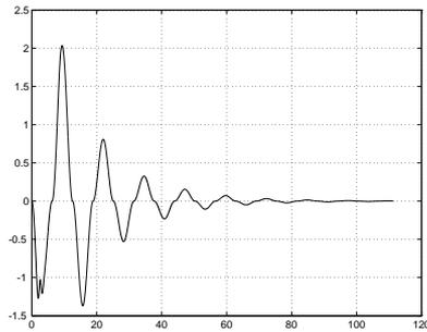
**Fig. 46.** Point stabilization with nonsmooth time-varying feedback (II):  $v_1$  (m/sec) vs. time (sec)
