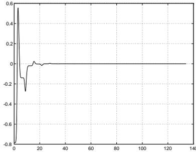
**Fig. 37.** Point stabilization with nonsmooth time-varying feedback (I):  $\theta$  (rad) vs. time (sec)
