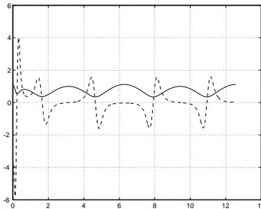
**Fig. 19.** Tracking an eight figure with a dynamic feedback linearization:  $v_1$  (—) (m/sec),  $v_2$  (---) (rad/sec) vs. time (sec)
