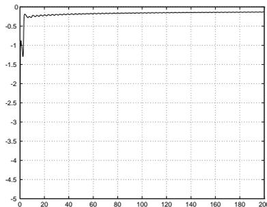
**Fig. 22.** Point stabilization with time-varying feedback and heat function  $\eta_2$ :  $y$  (m) vs. time (sec)
