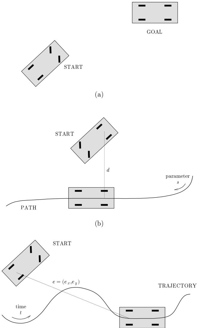
**Fig. 1.** Motion tasks: Point-to-point motion (a), Path following (b), Trajectory tracking (c)
