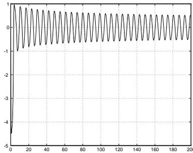
**Fig. 21.** Point stabilization with time-varying feedback and heat function  $\eta_2$ :  $x$  (m) vs. time (sec)
