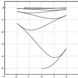
**Fig. 27.** Point stabilization with time-varying feedback and heat function  $\eta_4$ : cartesian motion
