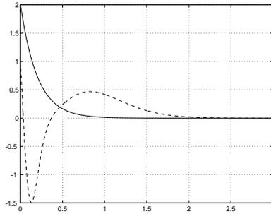
**Fig. 5.** Tracking a sinusoid with approximate linearization:  $x$  (—),  $y$  (---) errors (m) vs. time (sec)
