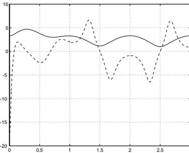
**Fig. 11.** Tracking a sinusoid with dynamic feedback linearization:  $v_1$  (—),  $v_2$  (---) errors (m/sec),  $v_2$  (---) (rad/sec) vs. time (sec)
