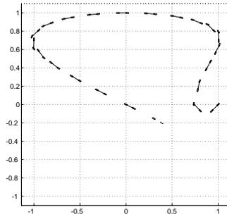
**Fig. 16.** Tracking an eight figure with dynamic feedback linearization: stroboscopic view of the cartesian motion
