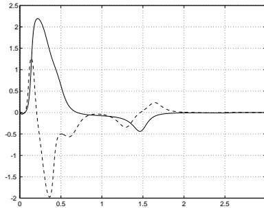
**Fig. 6.** Tracking a sinusoid with approximate linearization:  $\theta$  (—),  $\phi$  (---) errors (rad) vs. time (sec)
