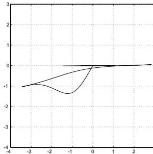
**Fig. 41.** Point stabilization with nonsmooth time-varying feedback (II): cartesian motion
