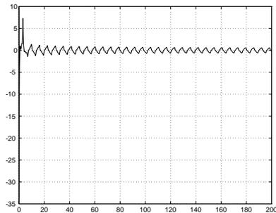
**Fig. 25.** Point stabilization with time-varying feedback and heat function  $\eta_2$ :  $v_1$  (m/sec) vs. time (sec)
