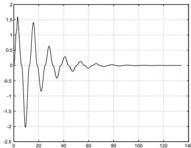
**Fig. 39.** Point stabilization with nonsmooth time-varying feedback (I):  $v_1$  (m/sec) vs. time (sec)
