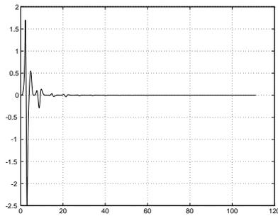
**Fig. 47.** Point stabilization with nonsmooth time-varying feedback (II):  $v_2$  (rad/sec) vs. time (sec)
