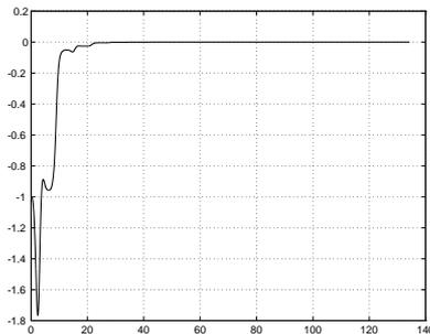
**Fig. 36.** Point stabilization with nonsmooth time-varying feedback (I):  $y$  (m) vs. time (sec)
