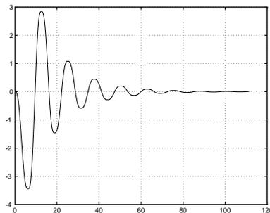
**Fig. 42.** Point stabilization with nonsmooth time-varying feedback (II):  $x$  (m) vs. time (sec)
