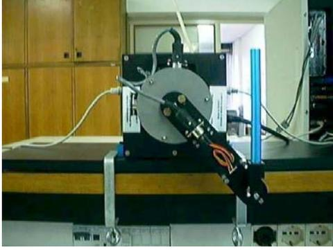
Fig. 1. The Quanser Pendubot used for experiments
