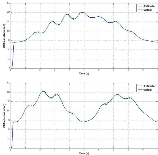
Fig. 8. On-line stiffness estimation for transmissions 1 (top) and 2 (bottom) of the VSA-II using the BBE strategy and the stability recovery scheme (33)
