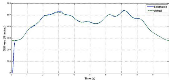
Fig. 9. On-line estimation of the *total* stiffness of the VSA-II device resulting from Fig. 8
