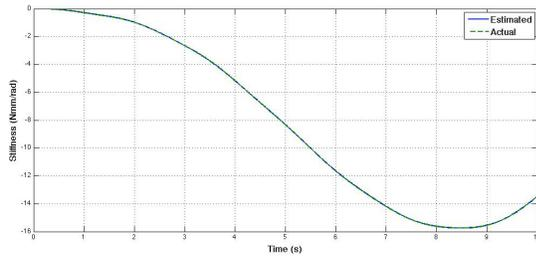
Fig. 1. Flexibility torque  $\tau_e$  for an elastic joint estimated during forced motion using the residual (14)
