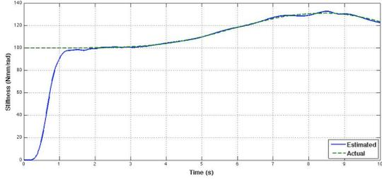
Fig. 5. On-line stiffness estimation for a joint with quadratic stiffness using the BBE strategy with the stability recovery scheme (33)
