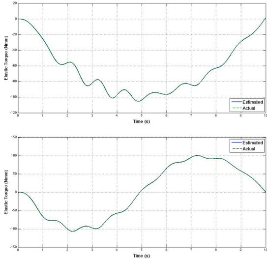
Fig. 6. Flexibility torques  $\tau_{e,1}$  (top) and  $\tau_{e,2}$  (bottom) for the VSA-II estimated during forced motion using two residuals as in eq. (14)
