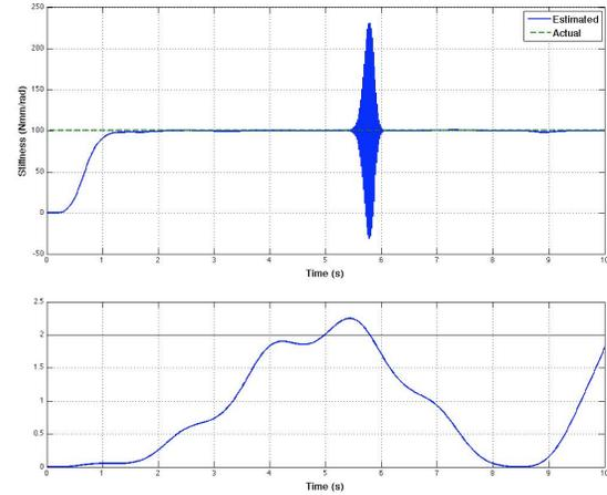
Fig. 2. On-line stiffness estimation for an elastic joint using the BBE strategy without the stability recovery scheme (top) and evolution of the dimensionless product  $K_R \dot{\phi}^2$  (bottom)
