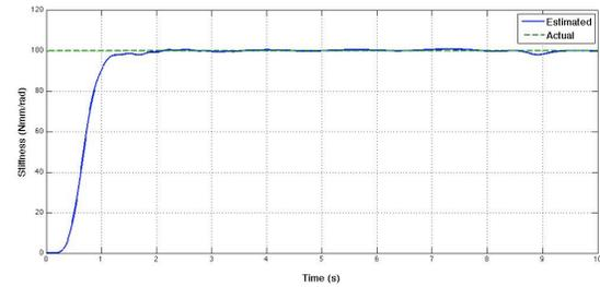
Fig. 3. On-line stiffness estimation for an elastic joint using the BBE strategy with the stability recovery scheme (33)
