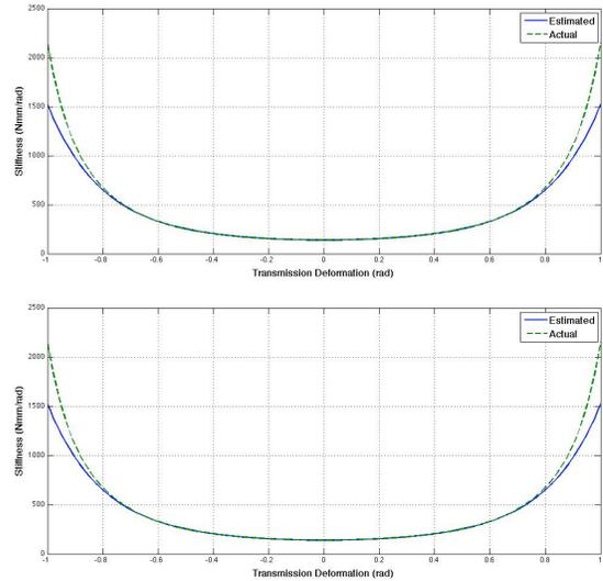
Fig. 7. Comparison of actual and estimated stiffness characteristics for transmission 1 (top) and 2 (bottom) of the VSA-II when using with the polynomial MBE strategy
