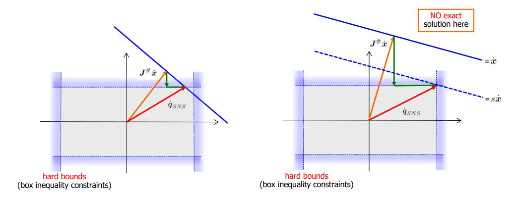
the total correction to the original pseudoinverse solution is always in the null space of the Jacobian (up to task scaling, if present)
