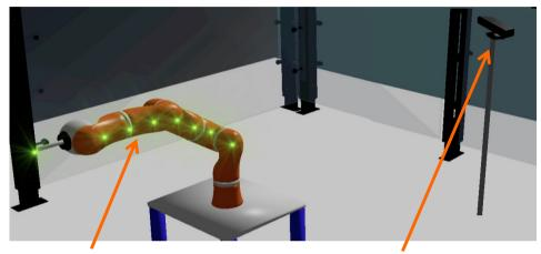
LWR4 robot with a finite number of control points a(q) (8, including the E-E)
