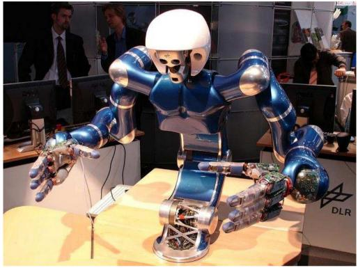
7R LWR-III lightweight manipulator: elastic joints (HD), joint torque sensing, 13.5 kg weight = payload
