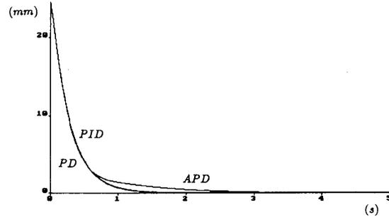
Fig. 1. End effector error: nominal payload = actual payload, initial error = 24 mm.
