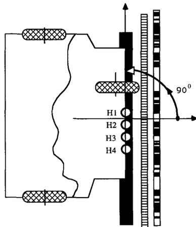
Fig. 8. AGV aligns its four reading heads on the guide-path and then turns 90° to reposition itself correctly on the guide-path.
