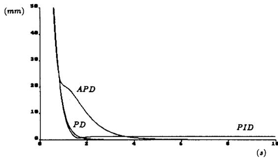
Fig. 2. End effector error: nominal payload = actual payload, initial error = 412 mm.
