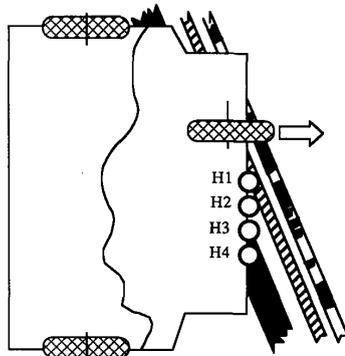
Fig. 7. AGV intersects the guide-path after avoiding an obstacle.
