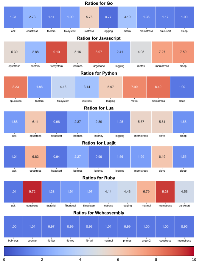
Fig. 7: CCA: ratios between mean execution times from secure and normal VMs for functions written in several languages.
