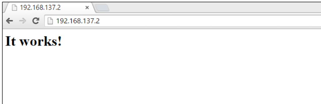
Figure 5-18. Apache2 providing a test web page
