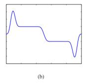
Fig. 4 Under/overshooting of the torque due to overconstraining boundary conditions
