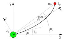
Fig. 1 A one-link planar flexible arm with definition of variables
