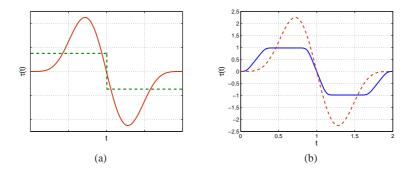
Fig. 2 (a) Polynomial torque for a flexible link vs. bang-bang torque (- -) for a mass-equivalent rigid link; (b) Polynomial torque vs. smoothed bang-bang torque (-) for the same flexible link
