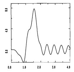
Figure 4. PD control (x-component of end-point error  $\times 10^{-2}$  ft).
