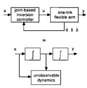
Figure 2. Closed-loop inversion control.
