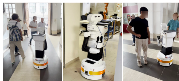
FIGURE 1 Snapshots of the TIAGo mobile manipulator, powered by the proposed sensor-based control framework, safely navigating multi-room environments populated by humans. Video: https://youtu.be/RYSQ3zmv30w .
