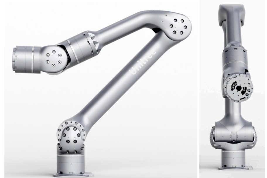
6-dof robot with a fully symmetric structure and an elbow offset
