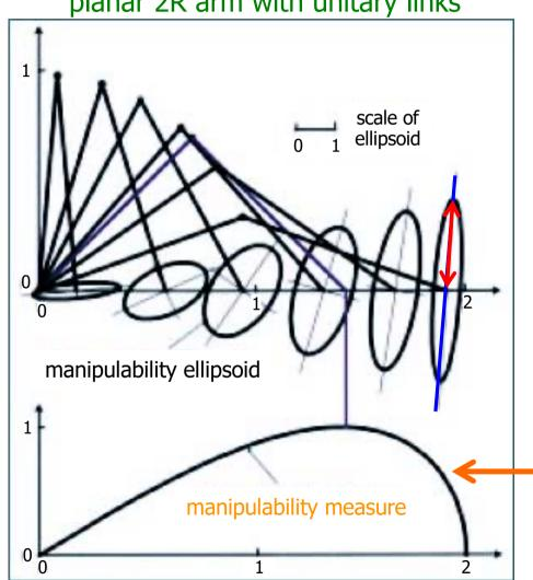
length of principal (semi-)axes singular values  $\sigma_i$  of I (in its SVD)
