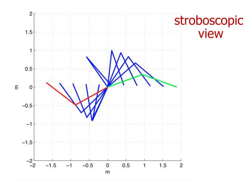
a line from right to left, at  $\alpha = 178^{\circ}$  angle with x-axis, executed at constant speed ||v|| = 0.6 m/s for T = 6 s
