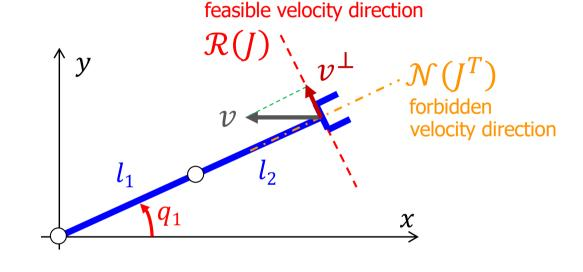
$\dot{q} = J^{\#}v$  is the minimum norm joint velocity vector that realizes exactly  $v^{\perp}$
