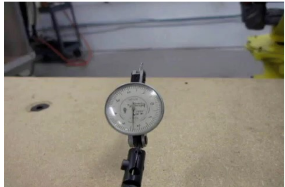
simple test on repeatability of a Fanuc ArcMate100i robot (1.3 m reach)
