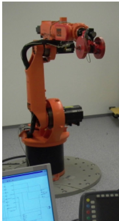
3-axis MEMS accelerometer on the forearm of a KUKA KR15/2 [DLR/Sapienza, 2007]
