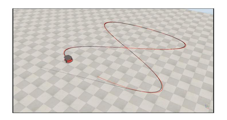
steady-state error is now reduced but steering velocity increases
