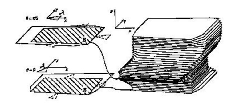
the  $\mathcal{C}$ -obstacle is obtained from the original obstacle via a "grow and stack" procedure
