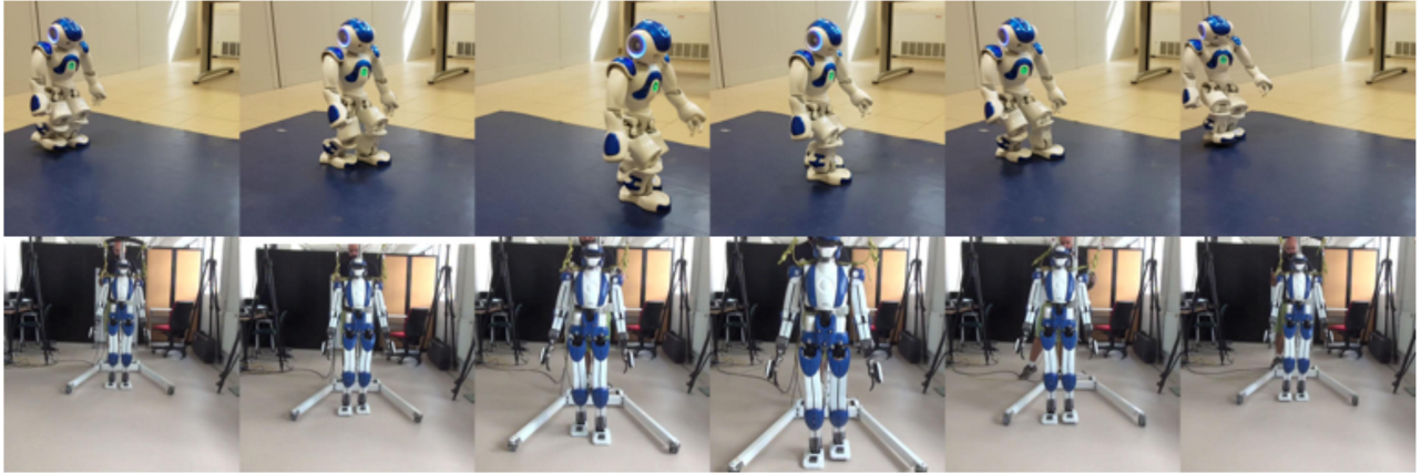
Fig. 20. Experiments 1 and 2: NAO and HRP-4 walking forward and backward. See the accompanying video.
