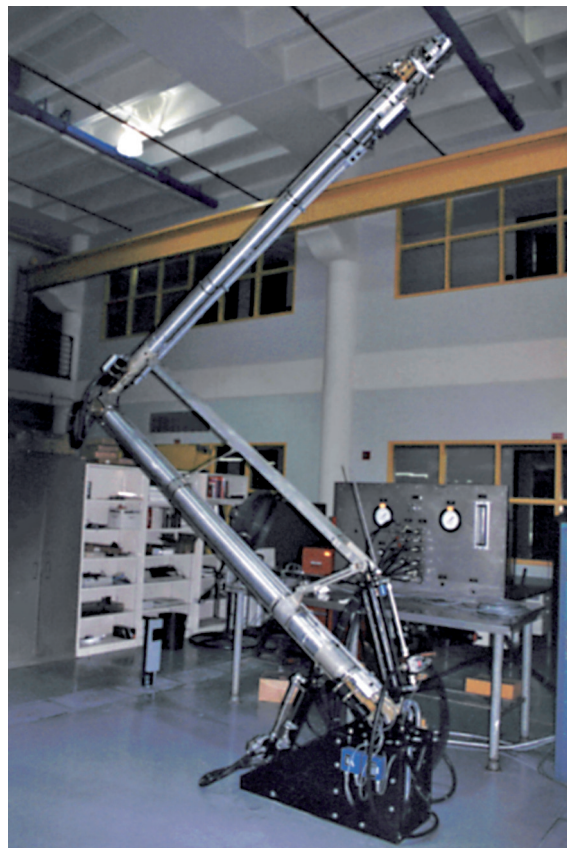
Fig. 13.15 Robotic arm large and flexible (RALF) used in EOA feedback experiments
