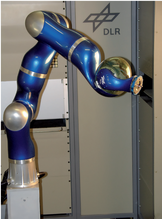
Fig. 13.3 The lightweight manipulator DLR LWR-III by the German Aerospace Center
