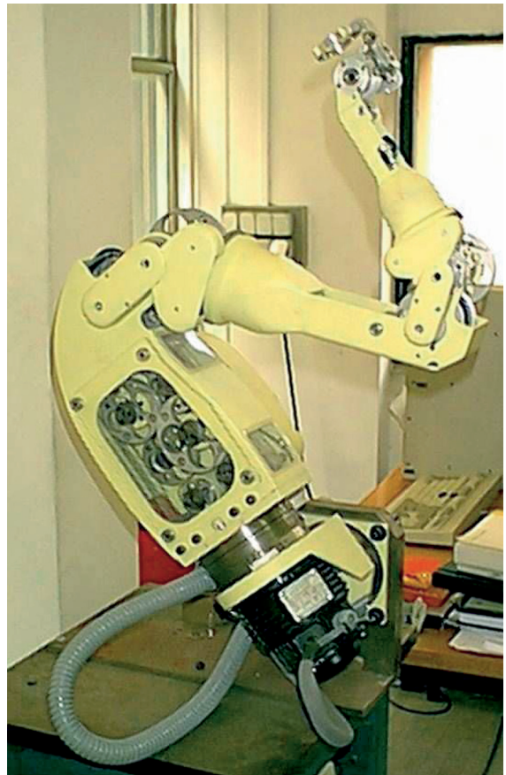
Fig. 13.2 The cable-driven robot Dexter by Scienza Macchinale
