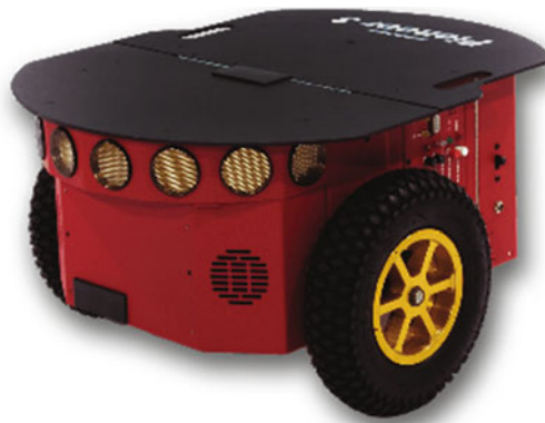
Fig. 1 The Pioneer by Adept is a popular differential-drive platform
