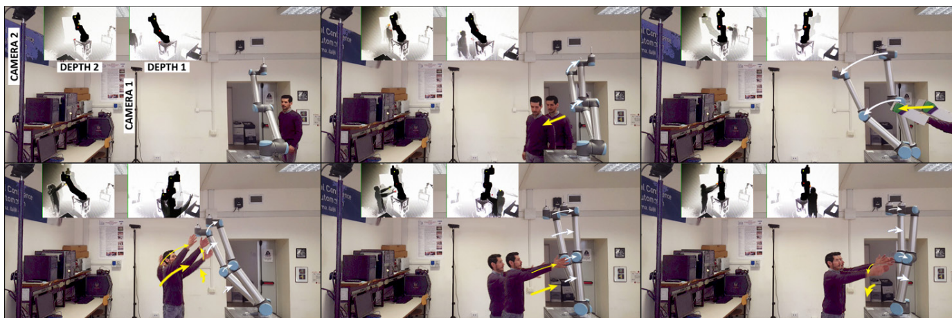
Fig. 5. Snapshots from an experiment. Yellow and white arrows indicate, respectively, the motion direction of the obstacles and of the robot.
