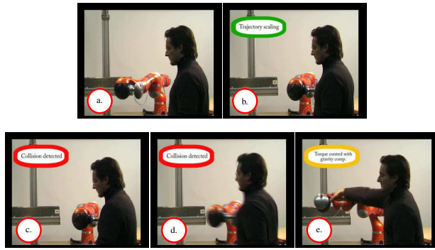
Fig. 7. Combining safety during the execution of a task and during a real collision: (a.) The robot moves position controlled along its desired trajectory. (b.) The robot slows down (trajectory scaling) and in the end stops after physical contact with the human. If the human would step aside the robot would continue to move along its desired trajectory. (c.) The human pushes harder against the robot and consequently the collision detection is triggered. (d.) The robot compliantly floats away in torque control with gravitation compensation (Strategy 2). (e.) Now, the robot can easily be moved around without being able to cause any harm.
