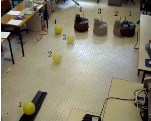
Fig. 12. A successful interception experiment with the ball traveling on a linear path. The numbers identify the position of the ball and the robot at four different time instants.
