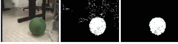
Fig. 3. Left : The image acquired by the camera. Center : After color recognition. Right : After noise filtering.
