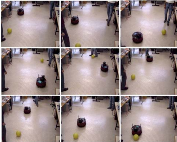
Fig. 13. An experiment where the robot tracks a ball passed back and forth by two human players
