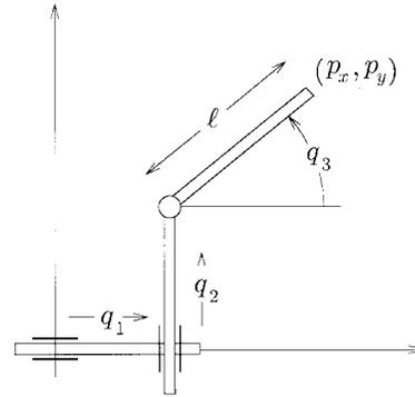
Fig. 1. A PPR planar robot.
