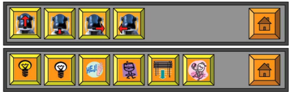
Fig. 8 The ASPICE GUIs for head control ( top ), and for vocal requests ( bottom )
