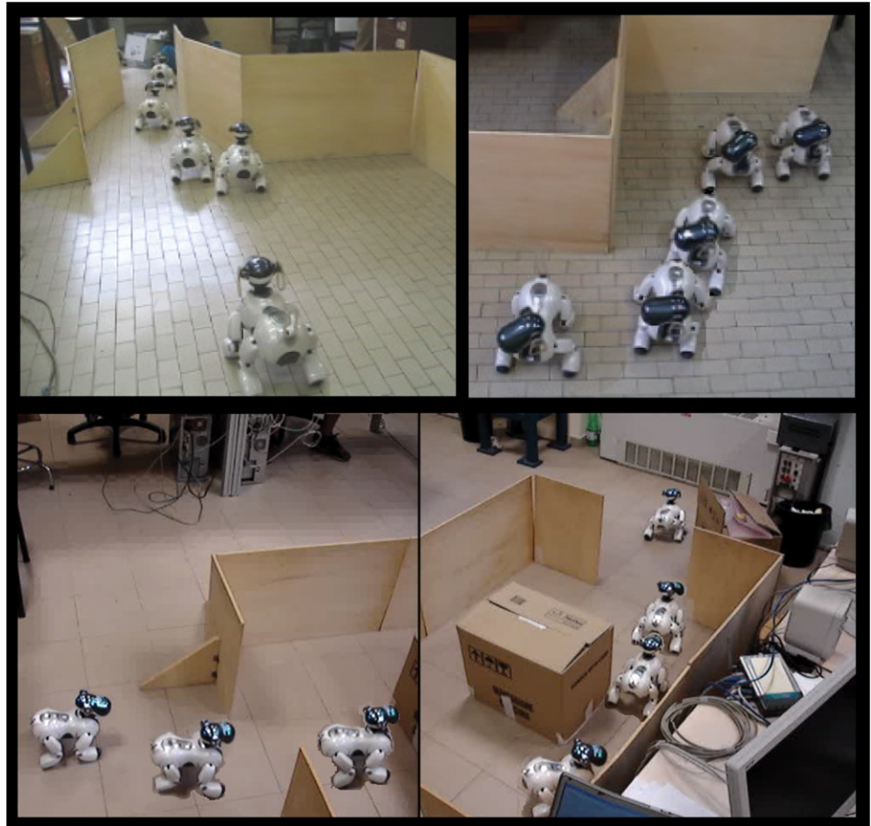
Fig. 10 Three experiments showing the performance of semi-autonomous navigation. The user drives the robot using a single command: ‘go forward’ ( top left and bottom ) and ‘go right’ ( top right )
