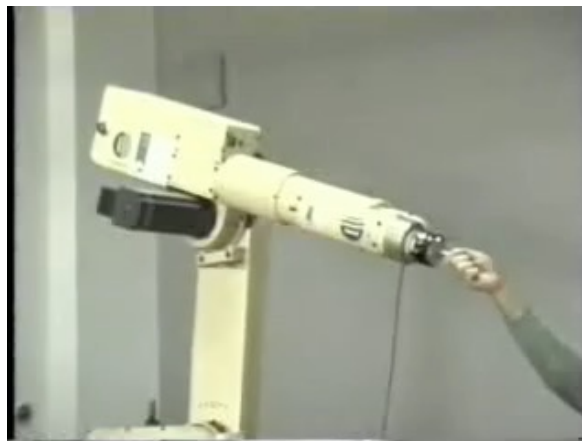
impedance control (with F/T sensor)
