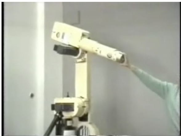
compliance control (active Cartesian stiffness control without F/T sensor)
