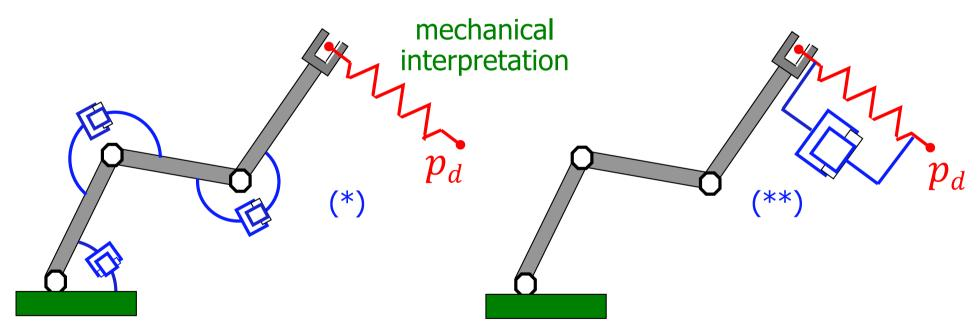
$J^T$  transforms the "virtual" elastic, for (\*), or visco-elastic, for (\*\*), force/torque acting on the end-effector into control torques at the joints
