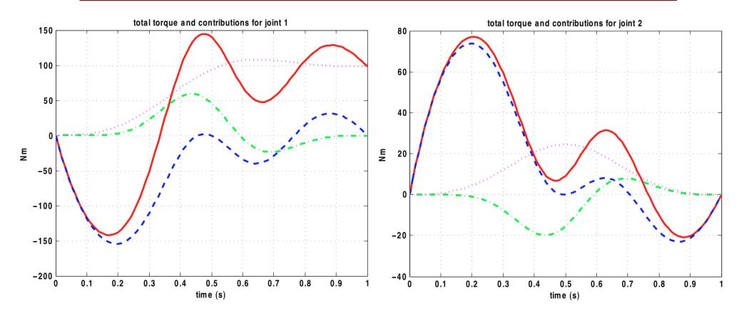
torque contributions at the two joints for the desired motion
