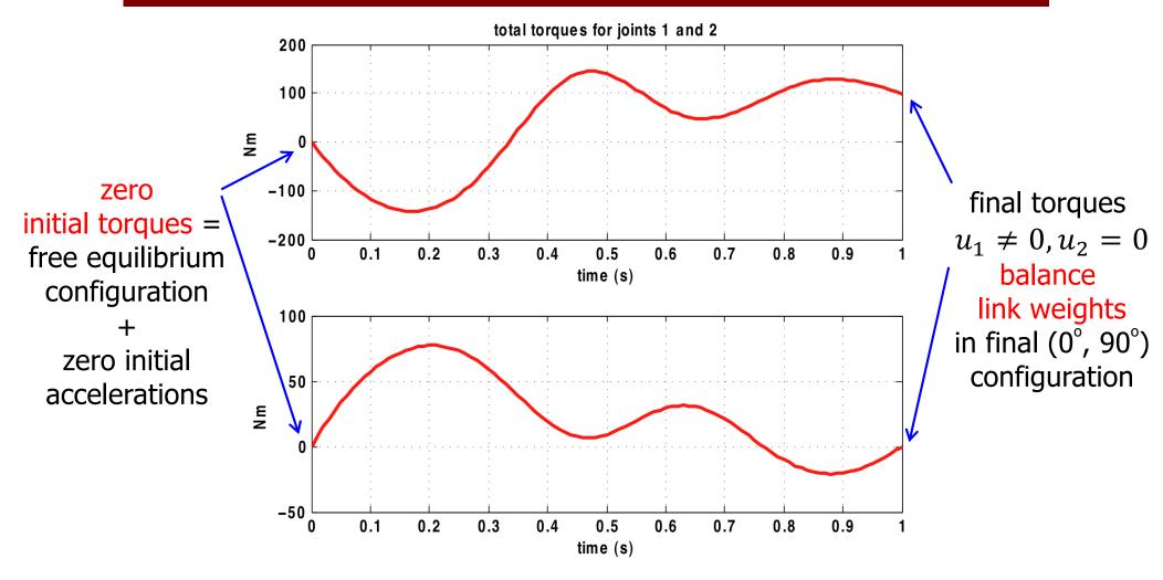
motion in vertical plane (under gravity) both links are thin rods of uniform mass  $m_1=10~{\rm kg},~m_2=5~{\rm kg}$
