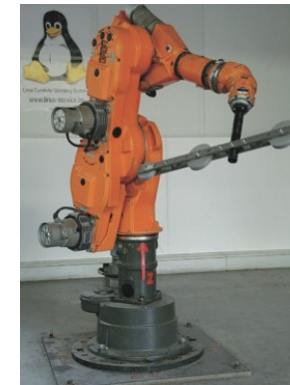
KUKA IR 361 robot and optimal excitation trajectory
