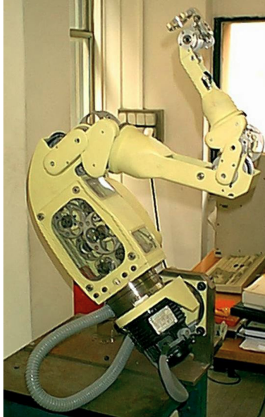
Dexter with cable transmissions
