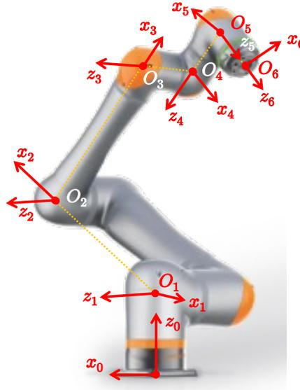
Figure 2: DH frames for the 6R robot Efort ECR5
