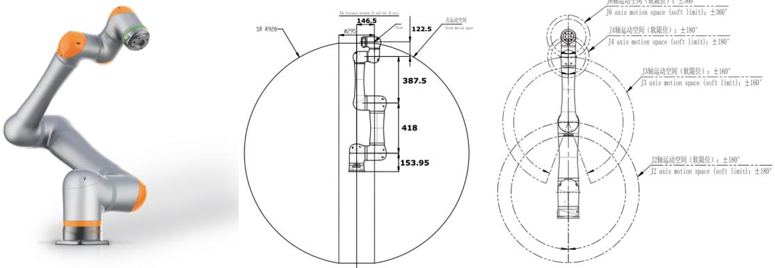
Figure 1: The 6R robot Efort ECR5 and drawings taken from the data sheet
