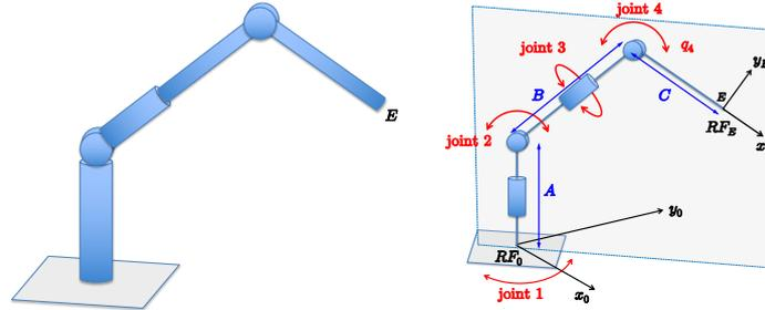
Figure 1: A 4R robot and its kinematic skeleton.
