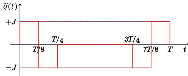
Figure 2: The jerk profile  $\ddot{q}(t)$  of the joint motion.
