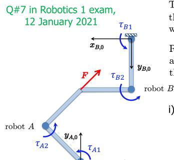
Two planar 2R robots A and B having unitary link lengths are in their D-H configurations  $\mathbf{q}_A = (3\pi/4, -\pi/2), \mathbf{q}_B = (\pi/2, -\pi/2)$  [rad] w.r.t. their base frames, as in figure (no gravity!).
