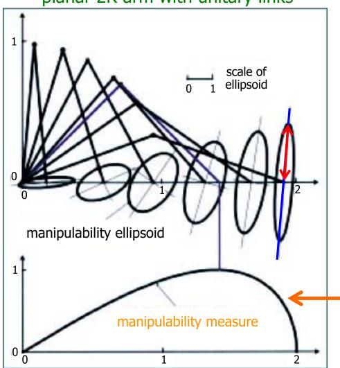
length of principal (semi-)axes singular values  $\sigma_i$  of J (in its SVD)
