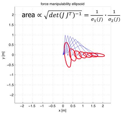
Cartesian **actuation** task (joint-to-task high transformation ratio): preferred velocity (or force) directions are those where the ellipsoid stretches
