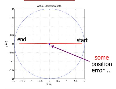
a line from right to left, at  $\alpha=179.5^\circ$  angle with x-axis, executed at constant speed v=0.6 m/s for T=6 s
