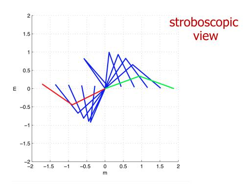
a line from right to left, at  $\alpha=178^\circ$  angle with x-axis, executed at constant speed v=0.6 m/s for T=6 s
