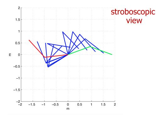
a line from right to left, at  $\alpha=170^\circ$  angle with x-axis, executed at constant speed v=0.6 m/s for T=6 s
