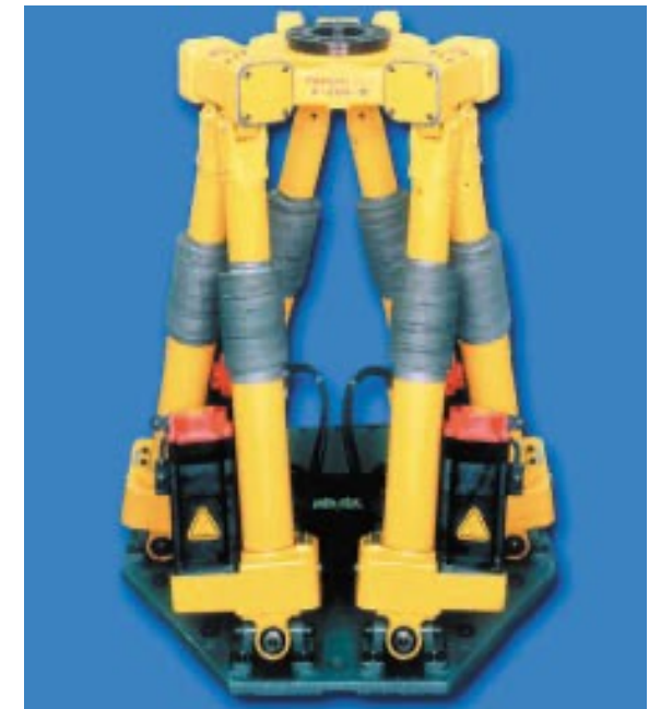
Fanuc F-200iB parallel kinematics
