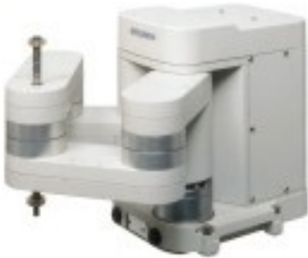
Mitsubishi RP (repeatability 5 micron, payload 5 kg)
