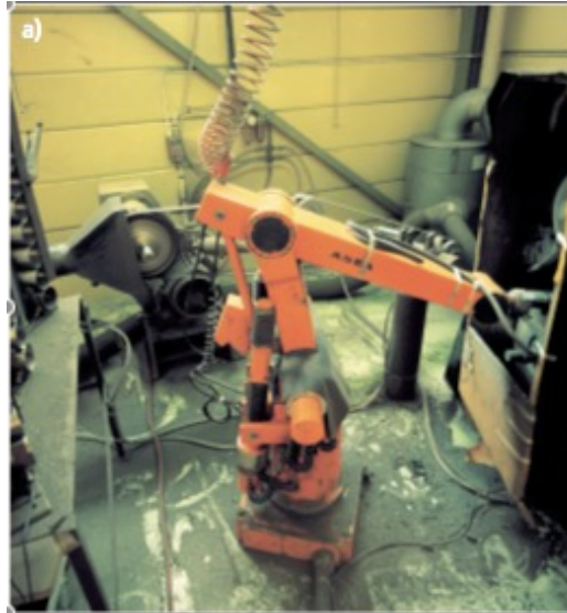
ASEA IRB-6 (1973) first robot all-electric-drives
