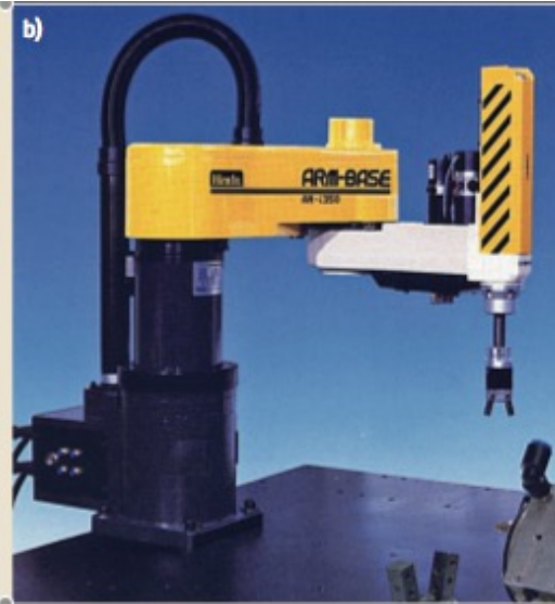
Hirata AR-300 (1978) first SCARA robot
