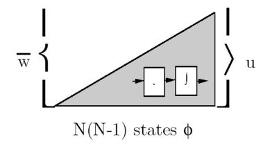
differentiate 2i times the component f<sub>i</sub> (i = 1,..., N) and apply a linear static control law (depending on K and S)
