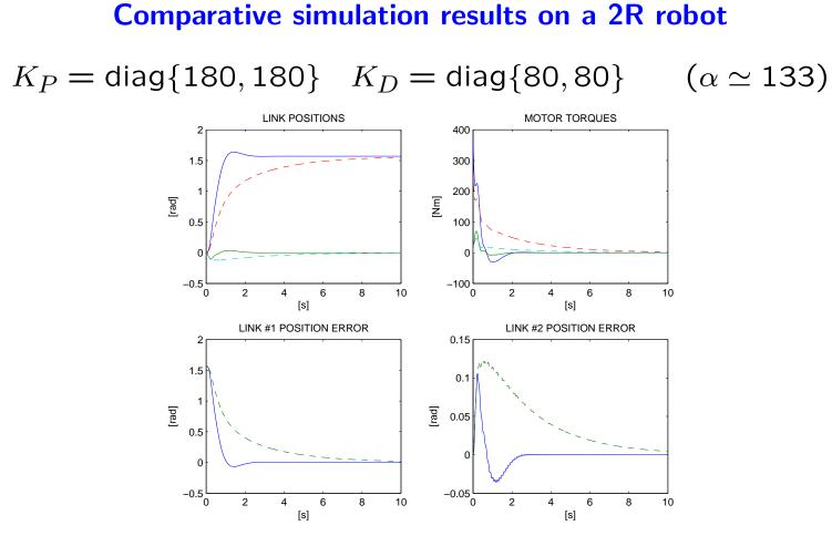
on-line (solid) vs. constant (dashed) gravity compensation
