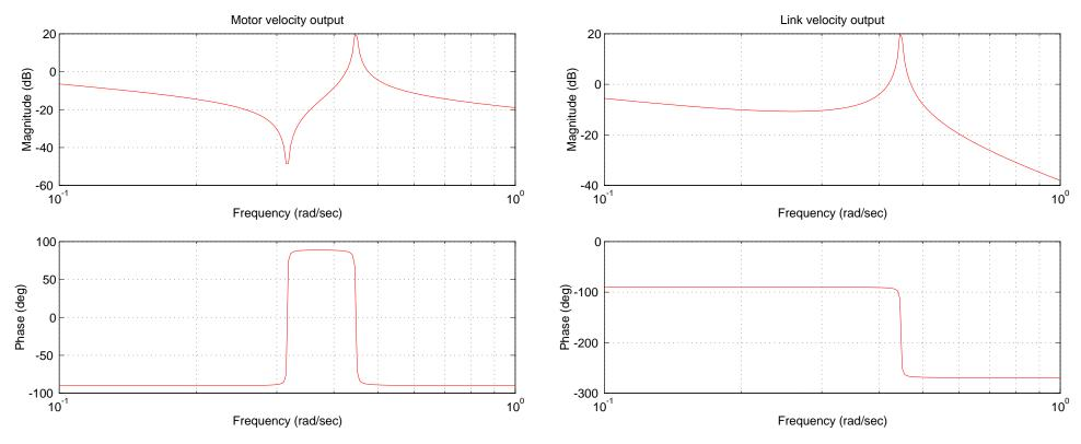
antiresonance/resonance behavior on motor velocity output, pure resonance on link velocity output (weak or no zeros)
