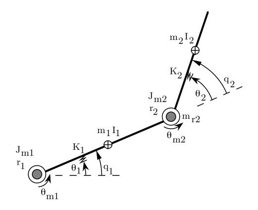
planar 2R arm with elastic joints (without or with gravity)
