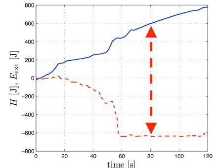
$$H(t) - H(t_0) = \int_{t_0}^t y^T u \, d\tau \underbrace{-\int_{t_0}^t \frac{\partial H^T}{\partial x} R(x) \frac{\partial H}{\partial x} d\tau}_{\leq 0}$$
