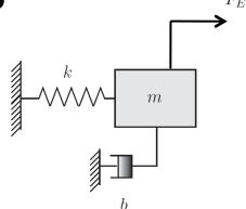
• This system was shown to be passive w.r.t. the pair (u, y) with u = f,  $y = \dot{x}$ , and as storage function the total energy (kinetic + potential)
