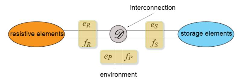
• An explicit example of a "Dirac structure" is the power-preserving interconnection represented by the skew-symmetric matrix J(x)
