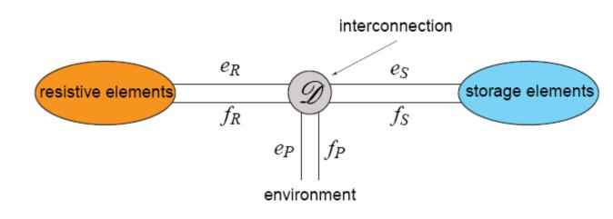
• A power port is a pair of variables  $(e,\,f)$  called "effort" and "flow" that mediates a power exchange (energy flow) among 2 physical components
