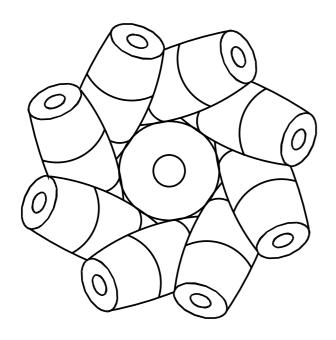
Mecanum (Swedish) wheels can be also used to build omnidirectional mobile robots
