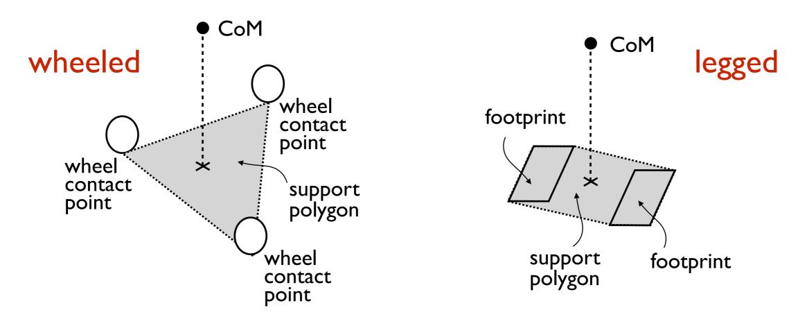
dynamical balance is a different type of balance in which the CoM is replaced by the Zero Moment Point (ZMP)
