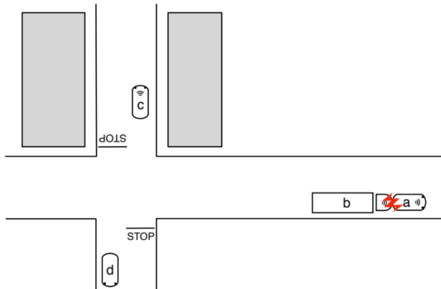
To prevent a collision, both truck *b* and car *a* must accelerate.
