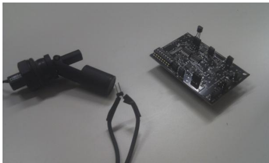
Figure 2 – (a) Temperature, liquid level sensors and event sensor board
