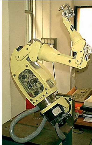
Dexter with cable transmissions
