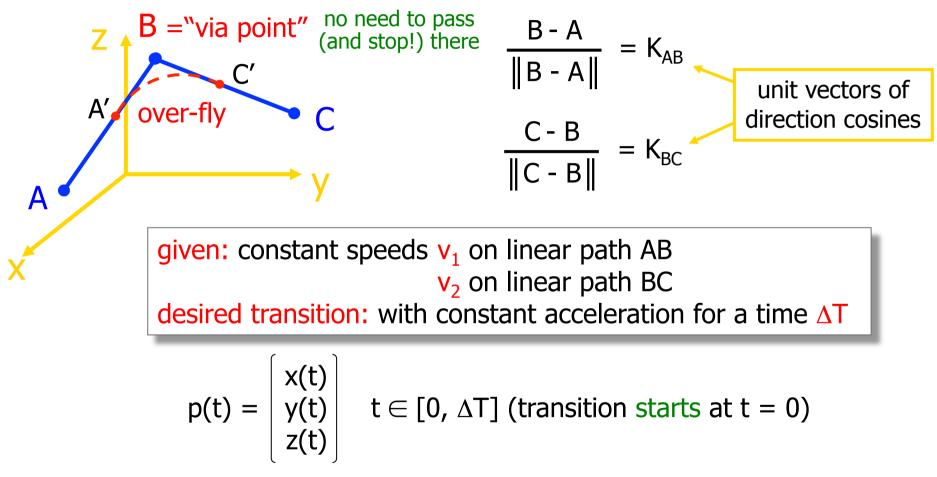
**note:** during over-fly, the path remains always in the plane specified by the two lines intersecting at B (in essence, it is a planar problem)
