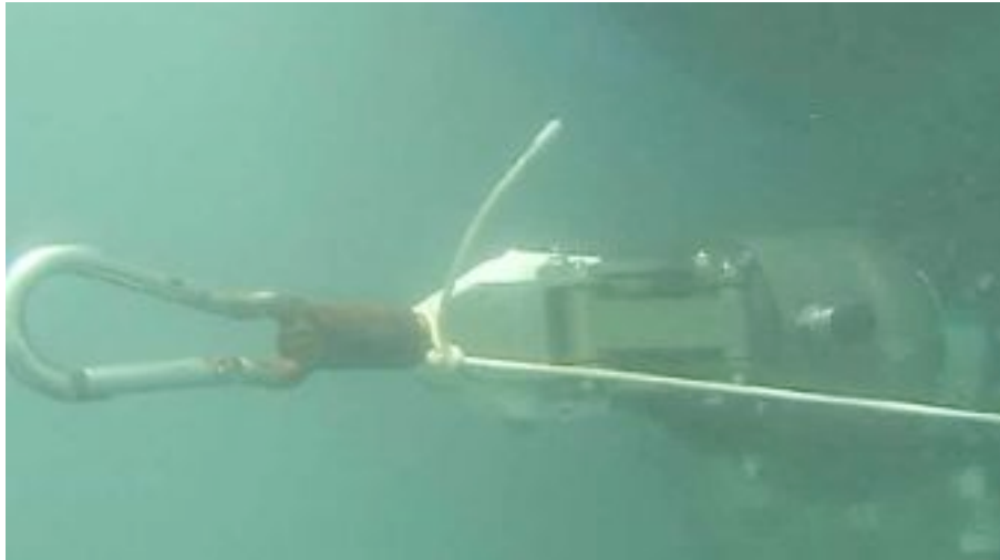
Ansaldo underwater arm performing a cable hooking task (SAUVIM project)
