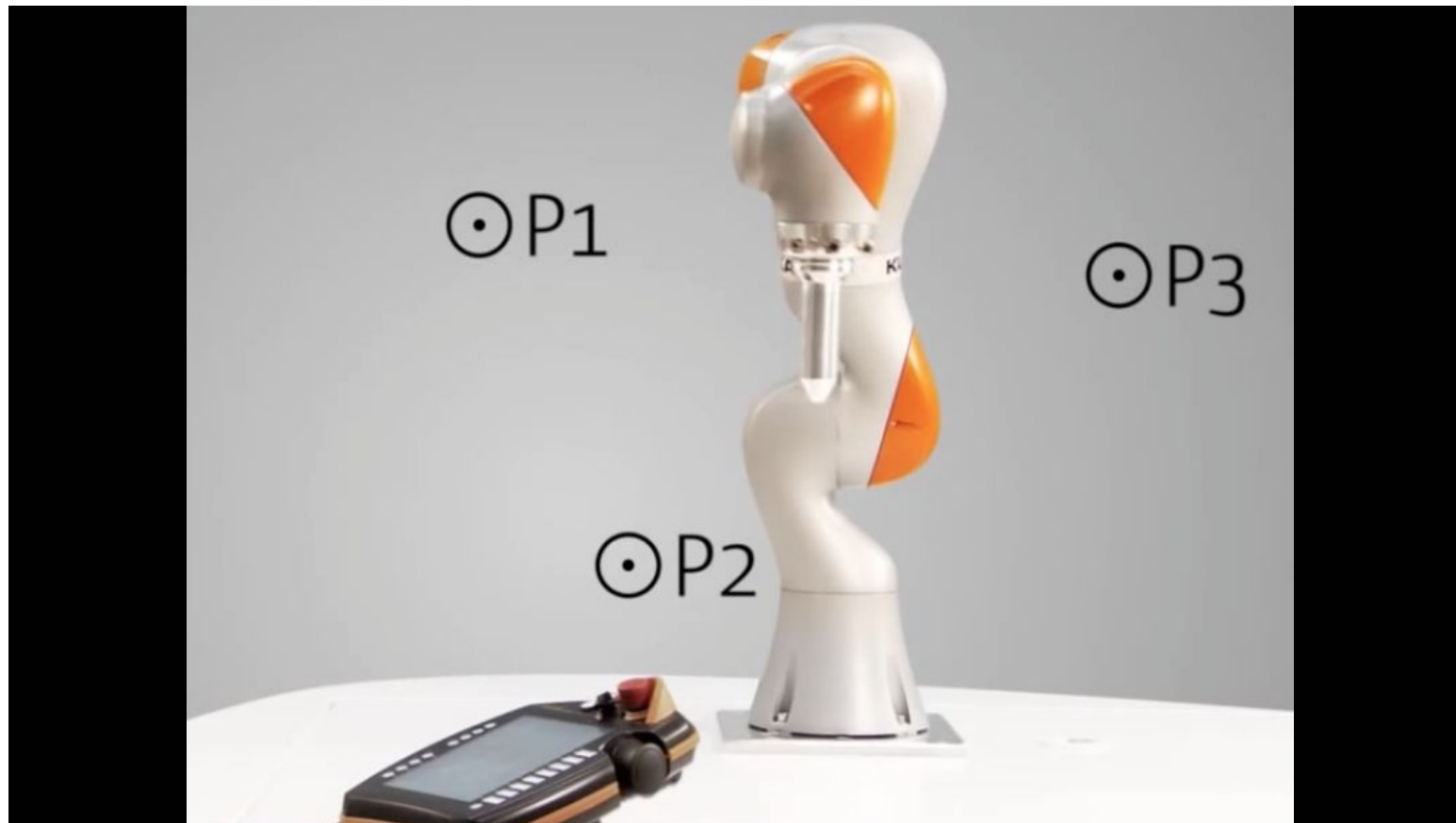
KUKA LBR iiwa robot with 7 revolute joints
