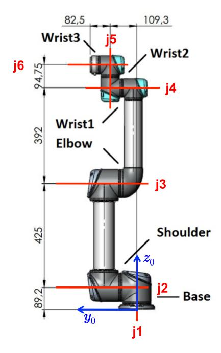
Draw all the Denavit-Hartenberg frames associated to the robot links according to Tab. 1 in the text.
