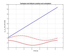
Figure 4: Cartesian position p(t) ( $p_x(t)$  [red],  $p_y(t)$  [red, dashed]) and angle  $\phi(t)$  [blue].
