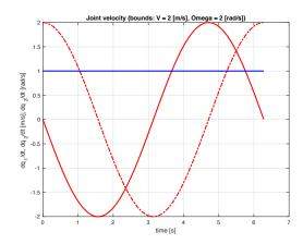
Figure 8: Joint velocity  $\dot{q}(t)$ :  $\dot{q}_1(t)$  [red],  $\dot{q}_2(t)$  [red, dashed],  $\dot{q}_3(t)$  [blue].
