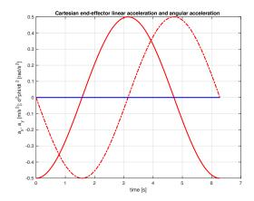
Figure 6: Cartesian linear acceleration  $\ddot{p}(t)$   $(a_x(t) \text{ [red]}, a_y(t) \text{ [red, dashed]})$  and angular acceleration  $\ddot{\phi}(t)$  [blue].
