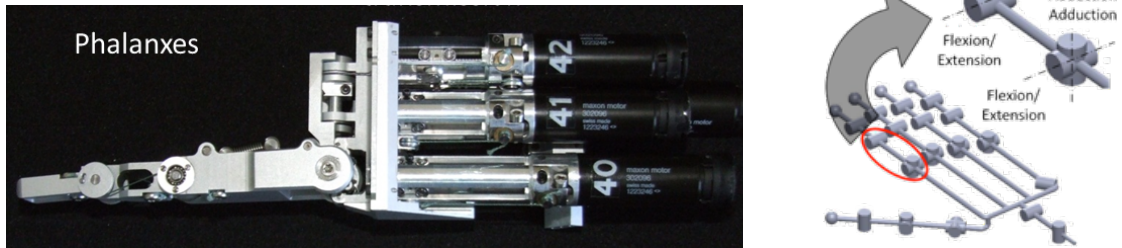
Figure 1: A 4-DOF finger of a robotic hand (left) and the kinematics of the full hand (right). The first three DOFs of the index finger are circled in red
