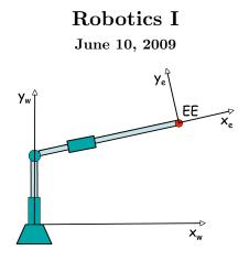
Consider the planar PRP robot with n = 3 joints in the figure above. The world reference frame  $RF_w = (\boldsymbol{x}_w, \boldsymbol{y}_w, \boldsymbol{z}_w)$  and the end-effector frame  $RF_e = (\boldsymbol{x}_e, \boldsymbol{y}_e, \boldsymbol{z}_e)$  are also shown.
